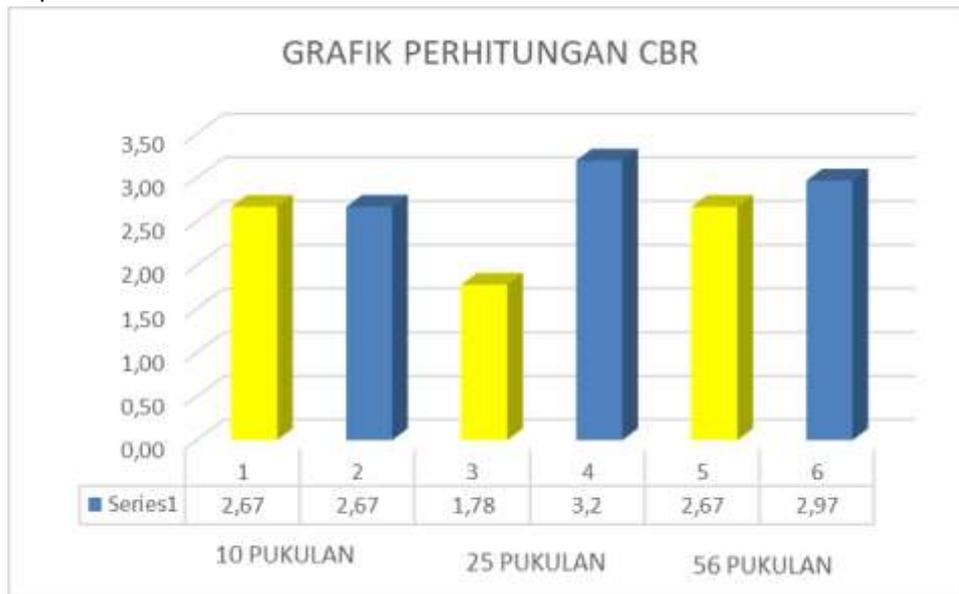
**Figure 4. 1** Graph of Soil CBR Calculation for 3 Trials
