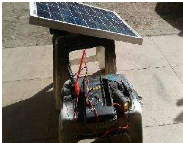
Figure 7. Solar Panel Measurement with 20 Watt Load
