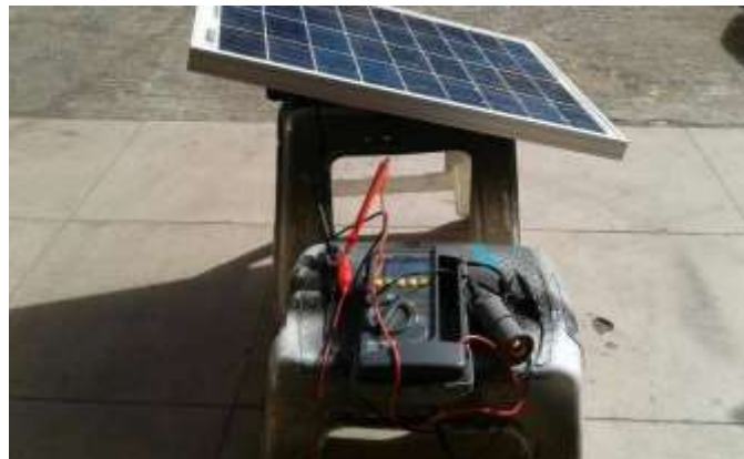
Figure 6. Solar Panel Measurement with 10 Watt Load
