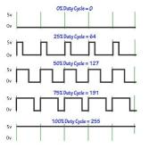
Figure 3. PWM waveform
