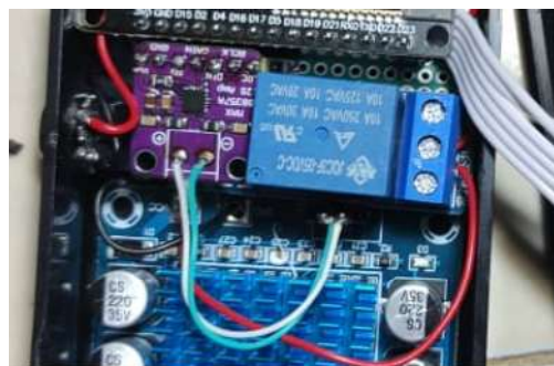
Figure 7. DAC pin configuration with ESP32 and amplifier, amplifier pins with speaker
