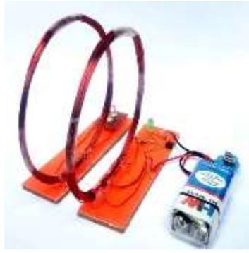
**Figure 9.** Wireless energy transfer research circuit
