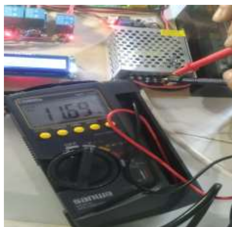
Figure 9. Power Supply Voltage Output Measurement
