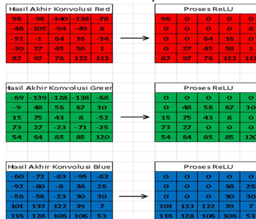
Figure 9. Final Result of RGB Convolution Sum and ReLU Process
